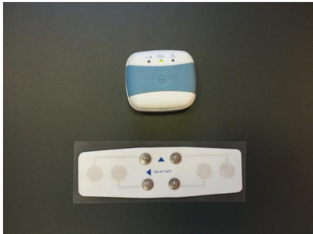
Figure 23: SPMHBGV3 wearable monitoring device and related B-Patch B-V3 patches.
