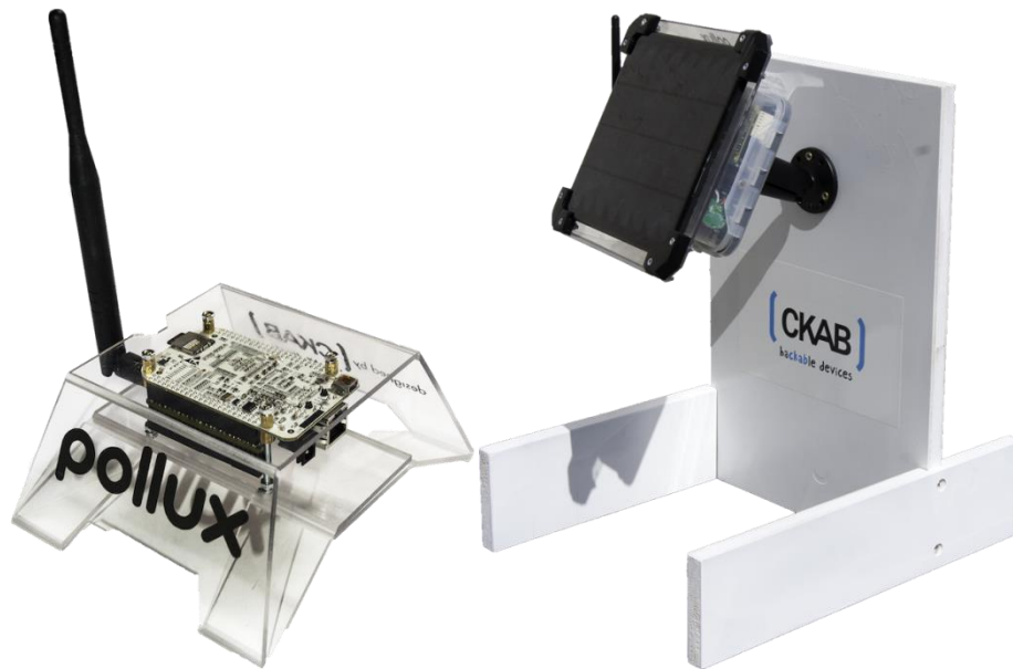
Figure 97: Pollux green station (gateway module and sensors)
