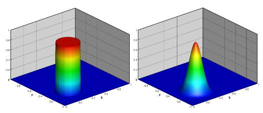
Figure 7: Discontinuous and continuous initial solutions in the coordinate system (x, y, u).
