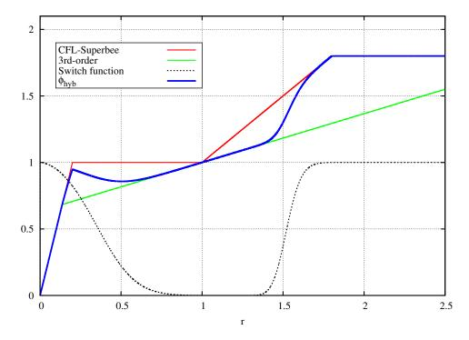
Figure 4: Switch function, pivots limiters, and hybrid limiter.
