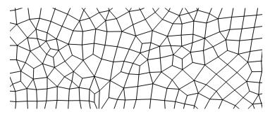
Figure 22: Sample of the hybrid unstructured mesh used for the Mach 3 wind tunnel test case.
