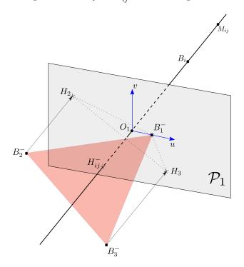
Figure 3: Illustration of the 3D algorithm to get the backward point  $\boldsymbol{H}_{ij}^{-}.$
