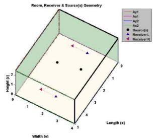
Fig. 3. The configuration of two microphone arrays and a pair of active speakers simulated using RoomSim [10].
