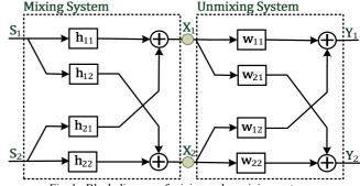
Fig. 1. Block diagram of mixing and unmixing systems.
