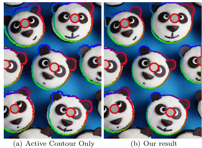
Fig. 7 Object contour extraction. (a) Object contour is extracted only using active contour. (b) Object contour is extracted using our method. The two leftmost occluded pandas are extracted through active contour, whereas the others are extracted by alpha matting
