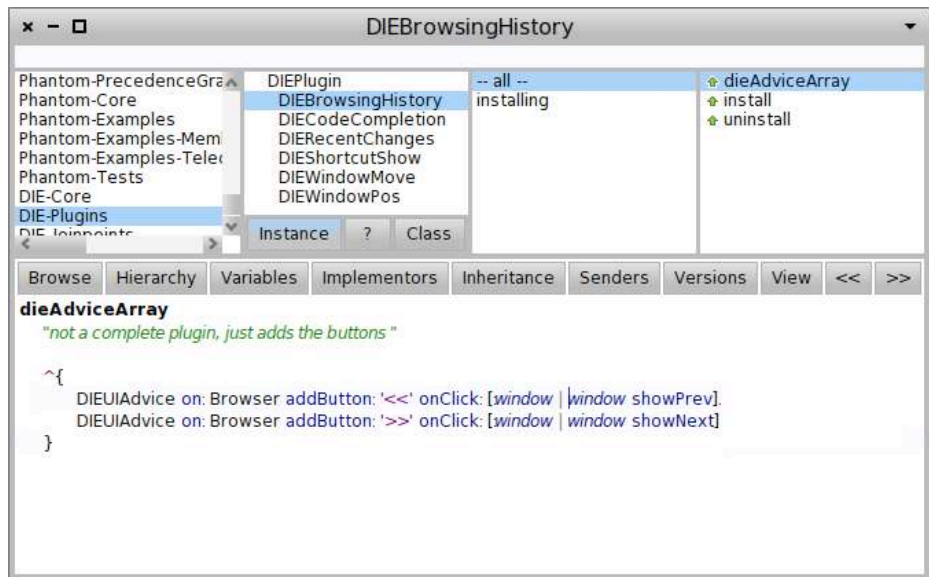
Figure 1: A DIE UI Advice inserting two buttons and the result: the last two on the right of the button bar.
