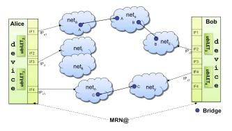
Fig. 4 Network-agnostic addressing over Multi-network overlay
