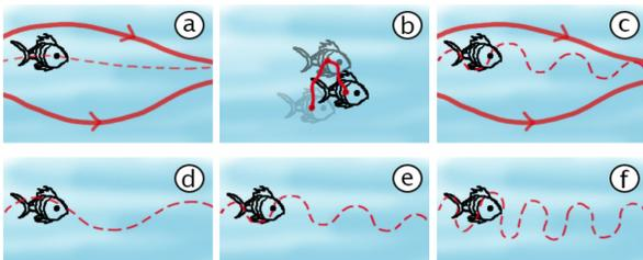
**Figure 6: Motion factorization. Combining (a) the global motion trajectory and (b) the granular motion results in (c) the trajectory of individual objects. Manipulating the velocity of granular motion affects the object's trajectory (d-f).**
