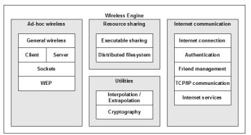
Fig.1: The Structure of the Network Engine.
