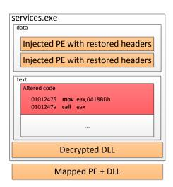
Figure 5. Memory space injected by Duqu into services.exe once the injection is done.
