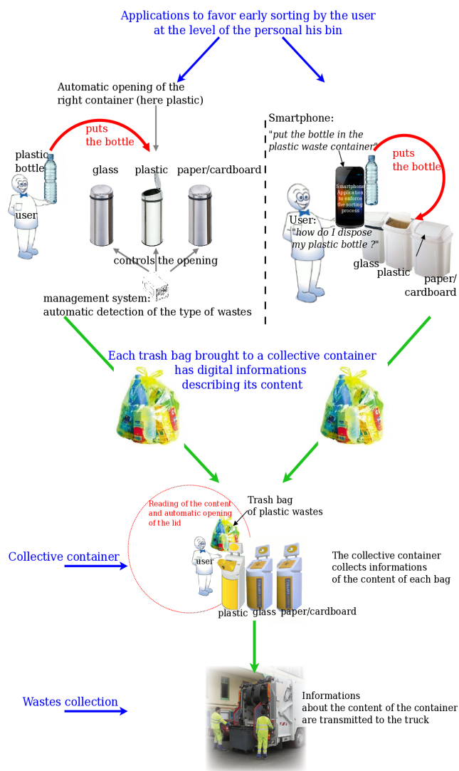
Figure 1. Waste flow and global architecture of the system.
