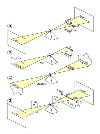
Fig. 3. A simple VE cell (a) representing the one-cell of maximal segments passing through vertex v and oriented edge e between blockers containing e's projections up and down. This VE cell is oriented and represented by the half-VE cell (b) and its opposite (c). A more complicated version (d) trimmed by occluders A and B demonstrates the need for also recording start and end edge endpoints.
