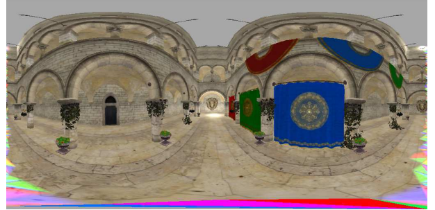
Figure 7: VE rendered with equirectangular projection. The triangles processed and clipped in the pre-clip stage are highlighted with colors. At the bottom, pole triangles are rendered with solid colors. At the left and right borders, rear triangles that were clipped are rendered with soft colors.
