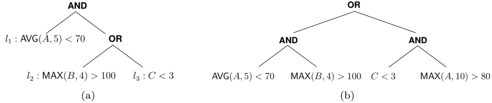
Figure 1. Two query tree examples: (a) a read-once query; (b) a shared query.
