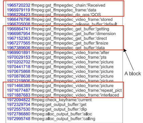
Fig. 6. A block in an execution trace
