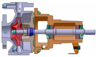
Figure 4 model of centrifugal pump.
