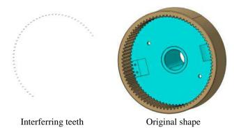
**Figure 9** Effect of rotational symmetry inaccuracies. Not all the teeth are interfering whereas the components are exactly coaxial (courtesy ANTECIM).
