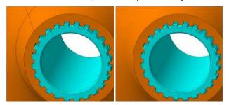
**Figure 10** Effect of maximal faces and edges generation. Patch boundaries are marked with black edges. Initial boundary decomposition (left), boundary decomposition with maximal faces and edges (right) (courtesy ANTECIM).
