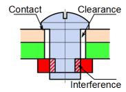
Figure 6 Geometric interactions of a bolt.
