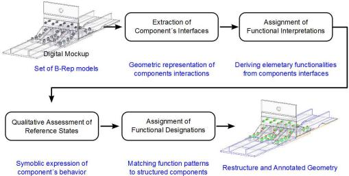
Figure 2 Overall scheme of processes
