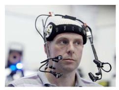
Figure 3 Head mounted camera system used to capture the facial expression of the actors.
