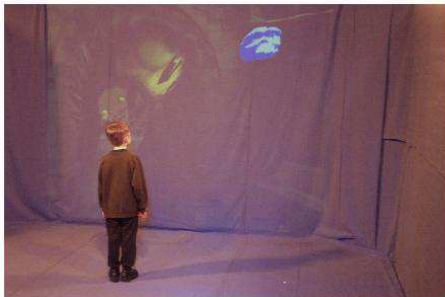
Figure 4: View-dependent projection on retro-reflective cloth
