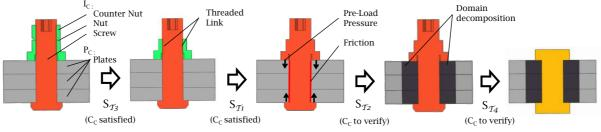
Fig. 6: Compatibility conditions (C<sub>c</sub>) of shape transformations  $S_{\tau}$  applied to T.
