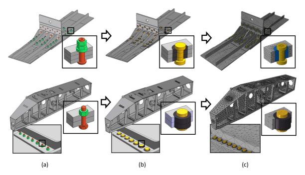
Fig. 11: (a) CAD model with functional designations and geometric interfaces, (b) model after applying  $S_{\sigma}(T)$  on bolts, (c) mesh assembly model with friction area definition.
