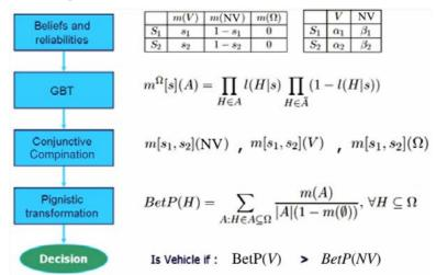
Figure 14 Fusion process for two sources
