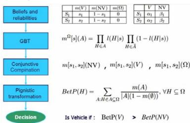
Figure 14 Fusion process for two sources
