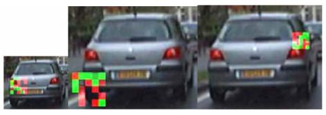
The genetic-like algorithm maintains a set of simple classifiers which are initialised as random ones. During each step of the algorithm, a new 'generation' of simple classifiers is produced by randomly applying some mutations (move, add or suppress a control point) on each of the simple classifiers. All of the mutations are tested and the one with the lowest error may replace the 'parent' if it has a lower error. In addition, some random simple classifiers are added at each step.
