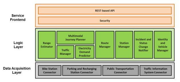
Figure 2: Software architecture of the Mobility 2.0 service backend
