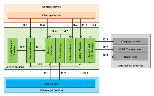
in Task 3.1 of Mobility 2.0, communication between clients and the server will be carried out over 3G. There will not be any direct communication between the vehicle and the nomadic device.
