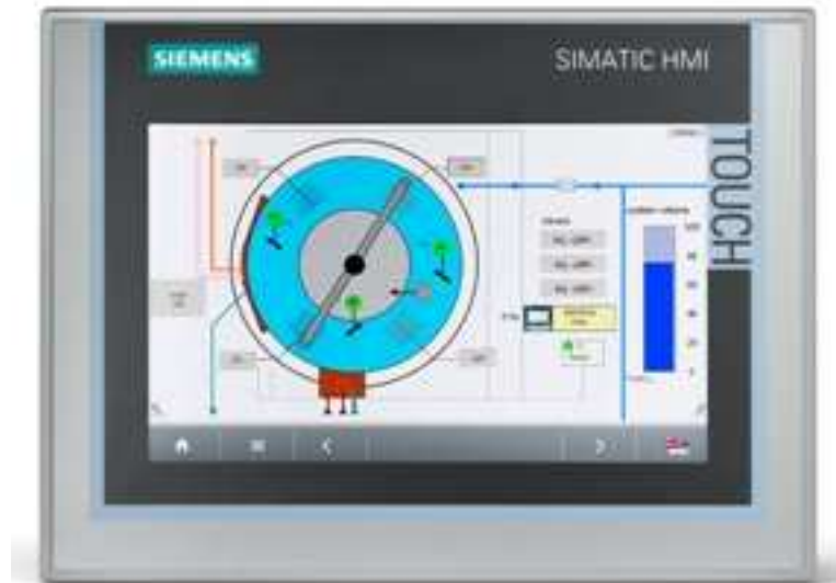
Figure 2.3: Simatic TP700 Comfort
