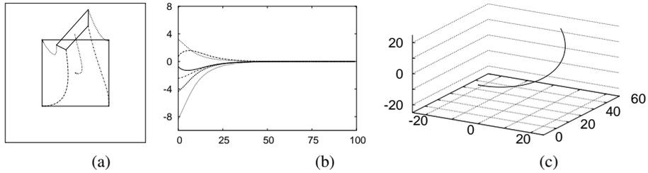
**Figure 6.18.** Servoing results when choosing  $\mathbf{s} = (x_1, y_1, \dots, x_4, y_4)$  and  $\mathbf{C} = \left( \frac{1}{2} \mathbf{L}_{\mathbf{s}} + \frac{1}{2} \mathbf{L}_{\mathbf{s}|\mathbf{s}=\mathbf{s}^*} \right)^+$
