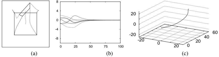
**Figure 6.16.** Servoing results when choosing  $\mathbf{s} = (x_1, y_1, \dots, x_4, y_4)$  and  $\mathbf{C} = \mathbf{L}_{\mathbf{s}}^+ |_{\mathbf{s}=\mathbf{s}^*}$
