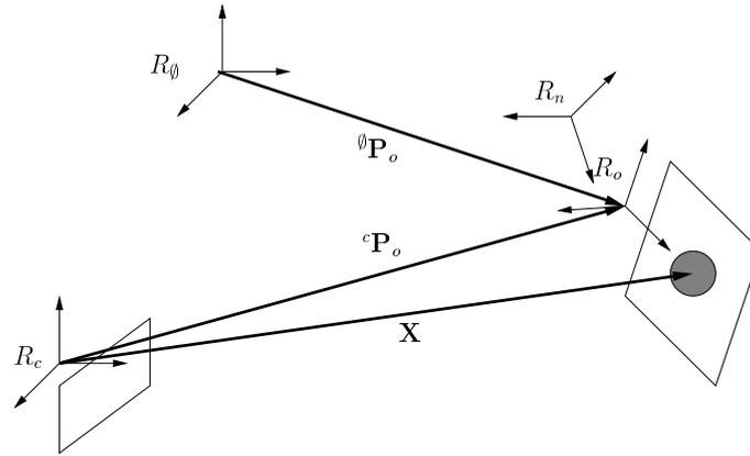
**Figure 6.8.** Possible 3-D points with a scene camera
