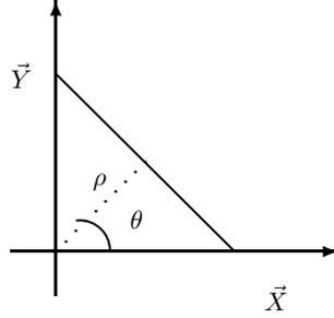
**Figure 6.5.**  $(\rho, \theta)$  representation of the 2-D lines
