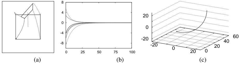
**Figure 6.11.** Servoing results when choosing  $\mathbf{s} = ({}^c\mathbf{t}_o, \theta\mathbf{u})$ : (a) trajectories of points in the image, (b) components of  $\mathbf{v}_c$  (in cm/s and deg/s) calculated at each iteration, (c) trajectory of the origin of the camera's frame in the frame  $\mathcal{R}_{c^*}$  (in cm)
