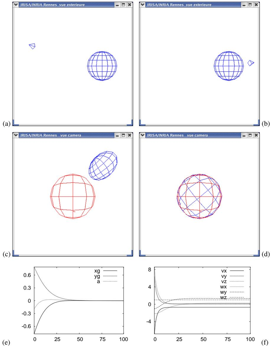
**Figure 6.21.** Positioning with respect to a sphere then movement around this sphere: (a) camera's initial pose with respect to the sphere, (b) camera's final pose, (c) superposition of the initial image and of the desired image, (d) superposition of the final image and of the desired image, (e) components of  $\mathbf{s}$  calculated at each iteration, (f) components of  $\mathbf{v}_c$  calculated at each iteration.
