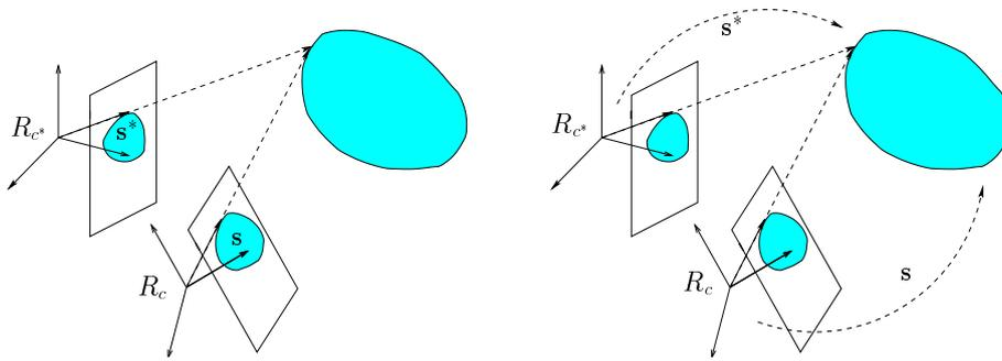
**Figure 6.1.** 2-D and 3-D visual servoing: 2-D visual servoing is used to bring the camera's frame of reference from  $R_c$  to  $R_{c^*}$ , based on measurements  $s$  extracted directly from the image (left). With 3-D visual servoing, the measurements  $s$  represent 3-D data estimated after an image processing phase (right).
