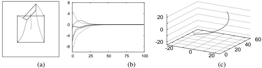
**Figure 6.17.** Servoing results when choosing  $\mathbf{s} = (x_1, y_1, \dots, x_4, y_4)$  and  $\mathbf{C} = \mathbf{L}_s^+$
