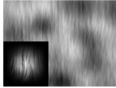
Figure 4: Sparse convolution noise. Lower left: windowed sample from an image of hair. Right: approximate hair texture created using 2D sparse convolution using this kernel.
