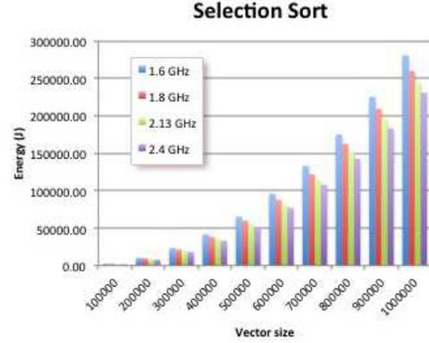
Fig. 3. Measured power consumption of the selection sort
