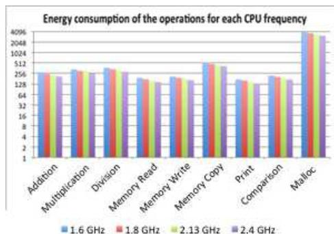
Fig. 2. Atomic power consumption of basis operations
