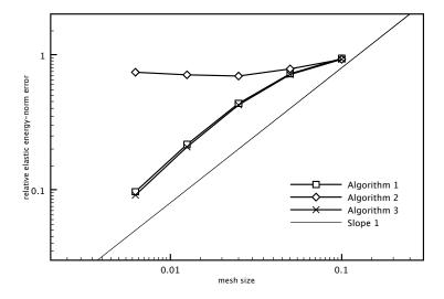
Figure 8: Implicit vs. explicit coupling. Convergence history of the displacement at time t = 0.015. Space-time grid refinement under  $\tau = \mathcal{O}(h)$ .
