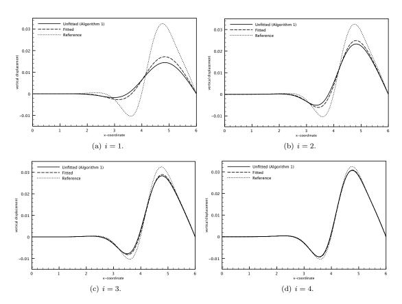
Figure 6: Unfitted vs. fitted methods. Comparison of the solid displacements at t = 0.015 for different levels of  $(\tau, h)$ -refinement, given by (33) with  $i = 1, \ldots, 4$ .
