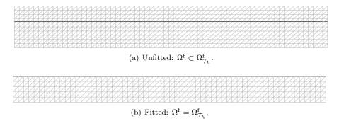
Figure 2: Computational fluid mesh (in grey) and solid domain (in black).
