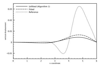
Figure 5: Comparison of the solid displacements at t = 0.015 obtained with  $\tau = 2 \cdot 10^{-4}$  and h = 0.1.
