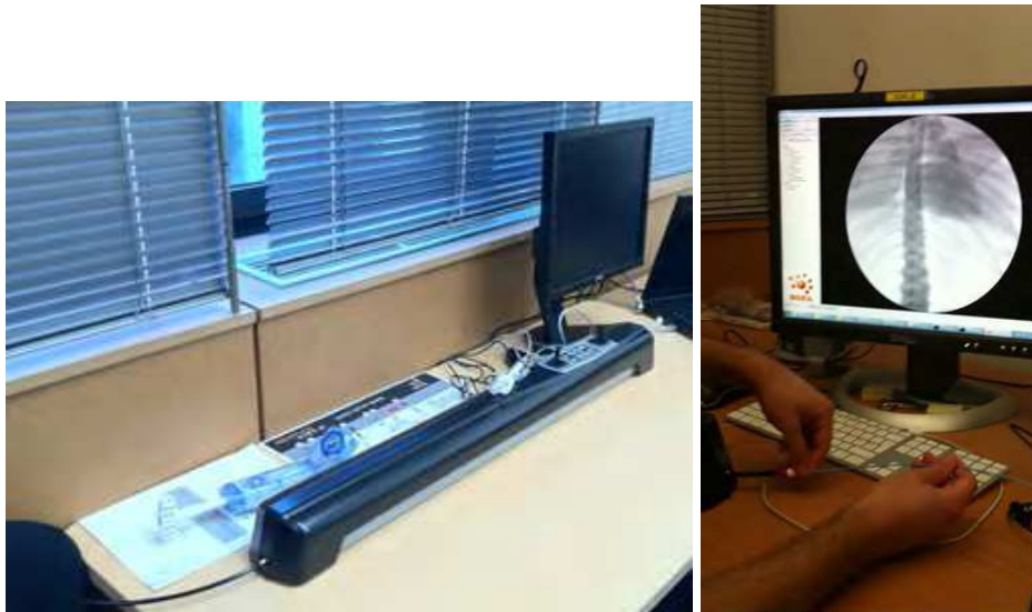
Figure 2: (Left) Hardware used to track up to three catheters and guidewires; (Right) Simulation hardware setup.
