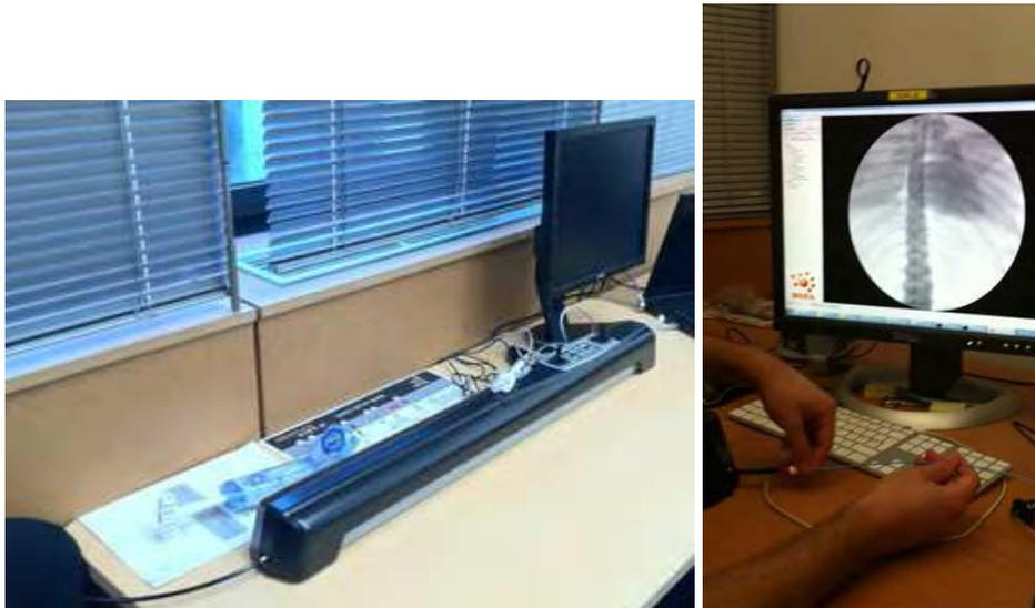
Figure 2: (Left) Hardware used to track up to three catheters and guidewires; (Right) Simulation hardware setup.
