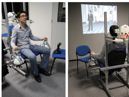
Figure 5: Experimental Setup, front view (left) and back view (right). The participant experiences haptic effects while watching a video.
