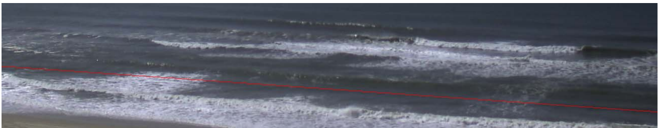
Figure 3. View from Truc Vert site. The red line is the timestack position. The timestack is parallel to the wave front.
