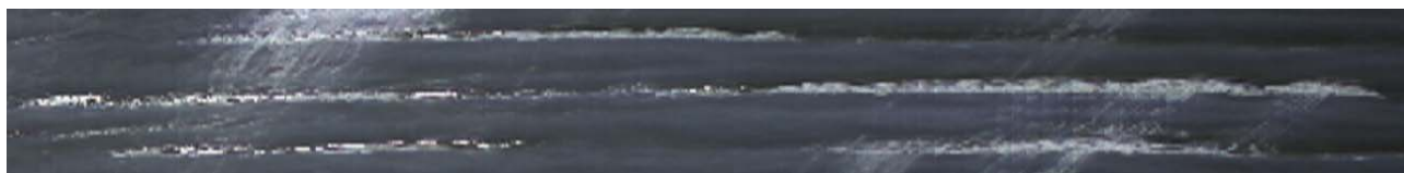
Figure 4. Associated timestack. The horizontal lines are wave crests. The orientation of the other lines created by the foam give the currents celerity along the shore.
