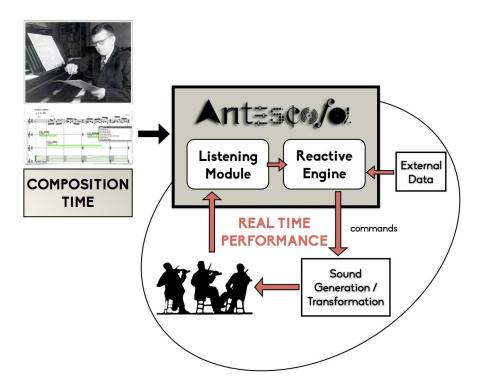
Figure 1: General architecture of *Antescofo*. The score is an input of both the listening machine and the reactive engine. The events recognized by the listening machine are signaled to the reactive engine which schedule the actions at the right time.
