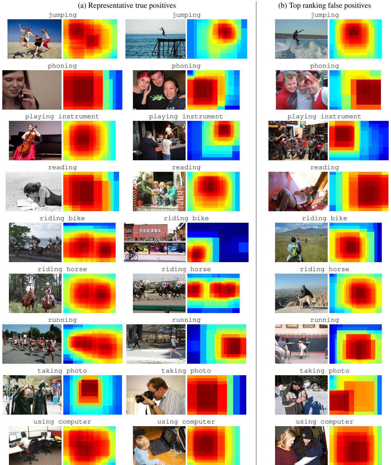
Figure 6: Representative high-scoring images and the corresponding response maps for the VOC 2012 action classification test set. Score maps provide estimates of action locations and scales in the image. The rightmost column contains the high-scoring false positive (according to our judgement) for each of the shown action categories. Please see additional results on the webpage of the project [2].
