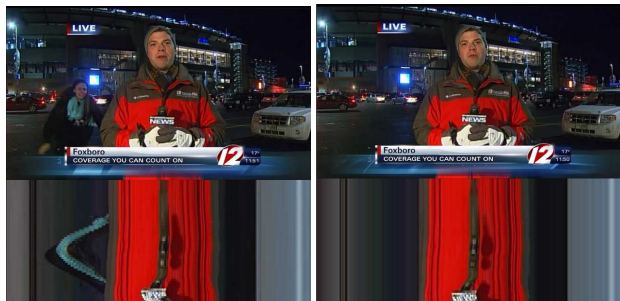
Figure 9. Inpainting task. Left : original video (top) and xt slice (bottom) showing trajectories. Right : our result (no artifact!). Clusters of fibers were computed and selected with only 7 mouse clicks to distinguish the disturbing girl from the reporter and background. The girl was removed and the hole was filled by extending the background fibers in time.
