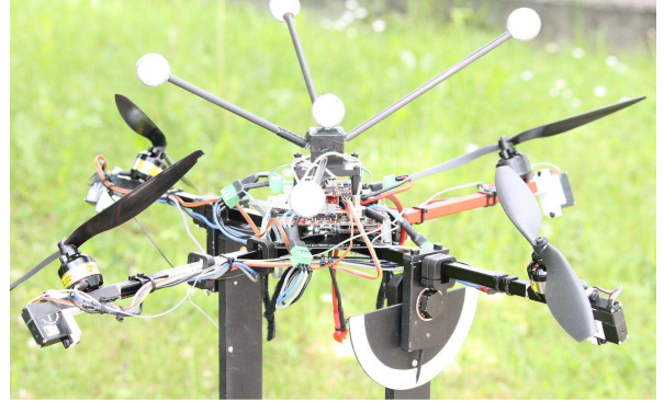
Fig. 1: A picture of the prototype on a testing gimbal
