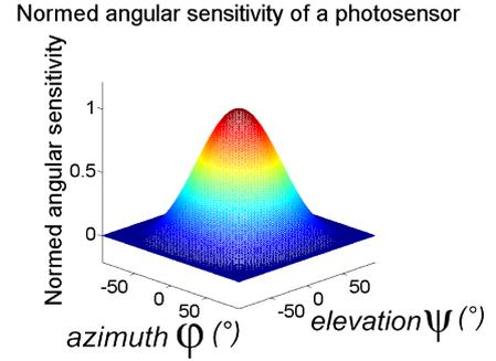
Fig. 3. Cosine-like angular sensitivity of a photosensor.
