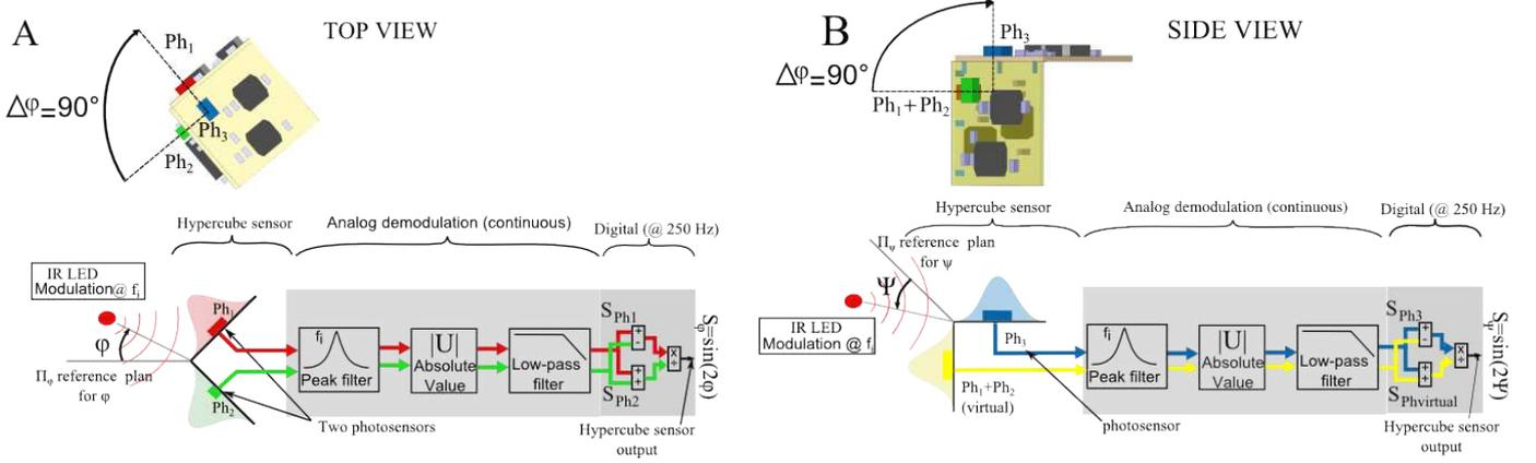
Fig. 5. Sketch diagram of HyperCube signal processing algorithm.
