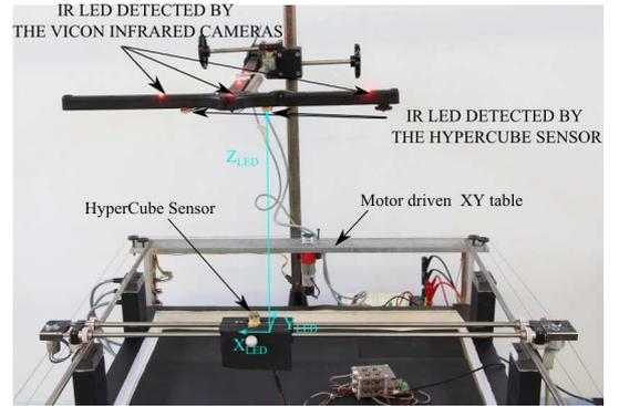
Fig. 9. XY table driven by DC motors. The the HyperCube positions is controlled in closed-loop by means of two incremental encoders. The distance  $Z_{LED}$  was assumed here to be known and constant. Additional active VICON markers were used to compare the precision of HyperCube with the ground truth acquired from the VICON motion capture system.
