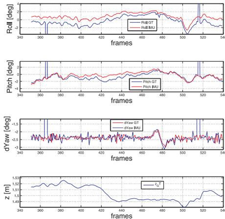
Fig. 12: From the top to the bottom: *Roll*, *Pitch* and *dYaw* angles [deg] estimated with the IMU (red) versus *Roll*, *Pitch* and *dYaw* angles [deg] estimated with the Optitrack system (blue). The last plot shows the height of the vehicle above the ground (non perfect planarity of motion).
