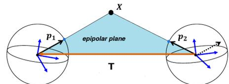
Fig. 3: Epipolar constraint.  $\mathbf{p}_1$ ,  $\mathbf{p}_2$ ,  $\mathbf{T}$  and  $X$  lies on the same plane (the epipolar plane).
