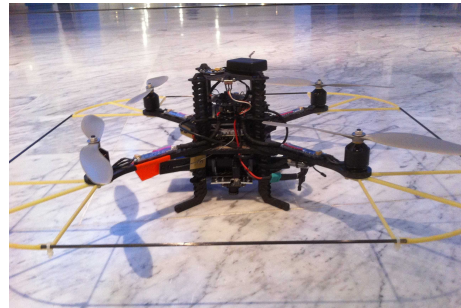
Fig. 1. AscTec Pelican quadcopter equipped with a monocular camera.
