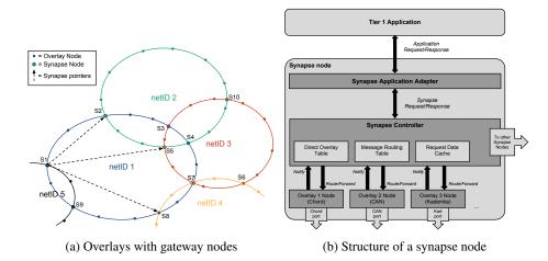
Fig. 1: Inter-overlay topologies and structure of synapse nodes
