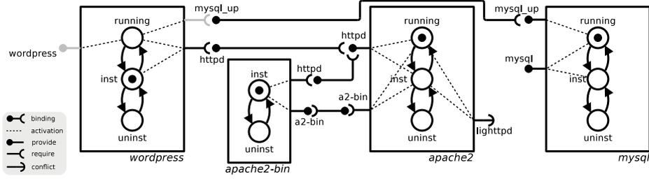
Fig. 1: Typical Wordpress/Apache/MySQL deployment, modeled in Aeolus core.
