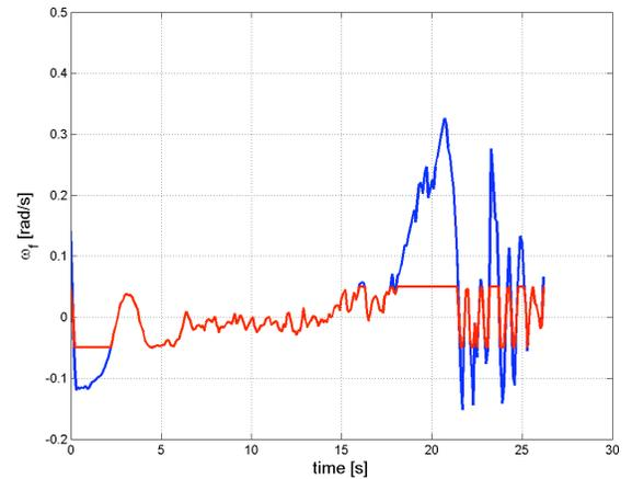
Fig. 25. The angular feedforward term  $\omega_{ff}$  without (blue line) and with (red line) saturation for the trajectory of Fig. 22
