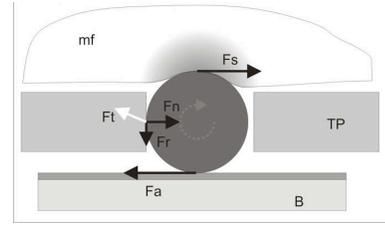
Fig. 13. Diagram of friction forces on a single ball. The ball is in contact with the shoe sole insisting with a mass  $m_f$ . When actuated, the belt applies a force  $F_a$  to the ball, which gets in point contact with the cylindrical hole of the supporting grid where forces  $F_n$  and  $F_r$  occur. The resulting force  $F_s$  is finally transmitted to the walker on the platform.
