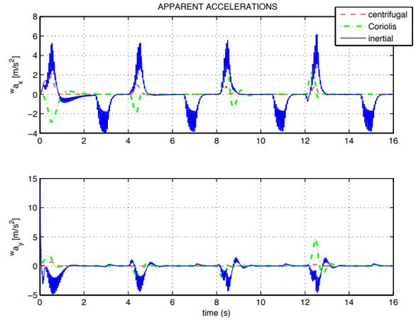
Fig. 10. Inertial, centrifugal and Coriolis components of the apparent acceleration felt by a user in the  $X_w$  (top) and  $Y_w$  (bottom) directions while walking along a square virtual path with acceleration control commands applied to the platform
