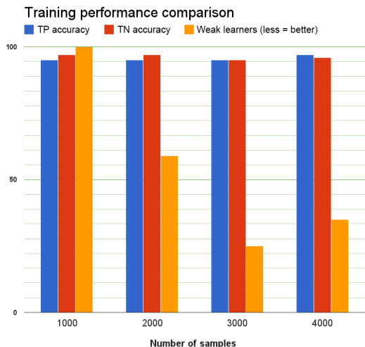
Figure 3: Random sampling training is performed with subsets of 1k, 2k, 3k and 4k size. The 3k subset (10.7% of parent set) reveals adequate discrimination and requires a low number of weak learners
