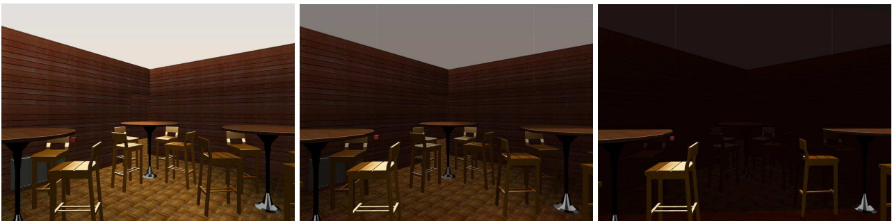
Fig. 5 Showing the location of the display screens of an immersive display to an immersed user to prevent him/her from hitting the walls. From the image on the left to the image on the right, the 3D visualization of the front screen evolves from being totally transparent to only 30% transparent as the user approaches with his/her hand (represented by the small red cube). The objects placed in front of the screen are not affected by this change, it makes the user aware of which objects can be reached safely by a physical move of his/her hand.
