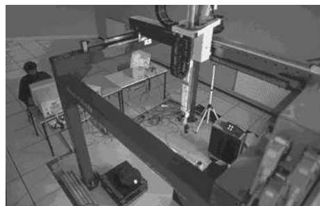
(a) Camera mounted on a 6 dof robot.
