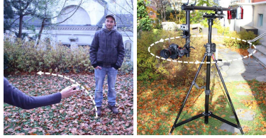
Figure 2. Our two capture setups: manually and using a motorised rotary stage.
