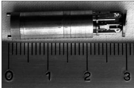
**Figure 1.4.** The MIPS micro-robot design for endoscopic surgery
