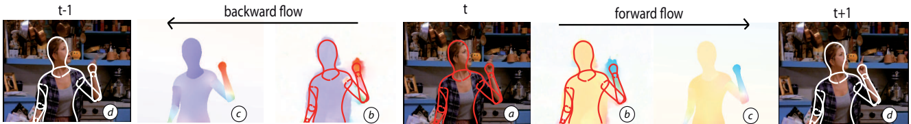
Figure 1. Flowing puppets. (a) Frame with a hypothesized human “puppet” model; (b) Dense flow between frame (a) and its neighboring frames; (c) The flow of the puppet is approximated by a part-based affine motion model; (d) The prediction of the puppet from (a) into the adjacent frames using the estimated flow.
