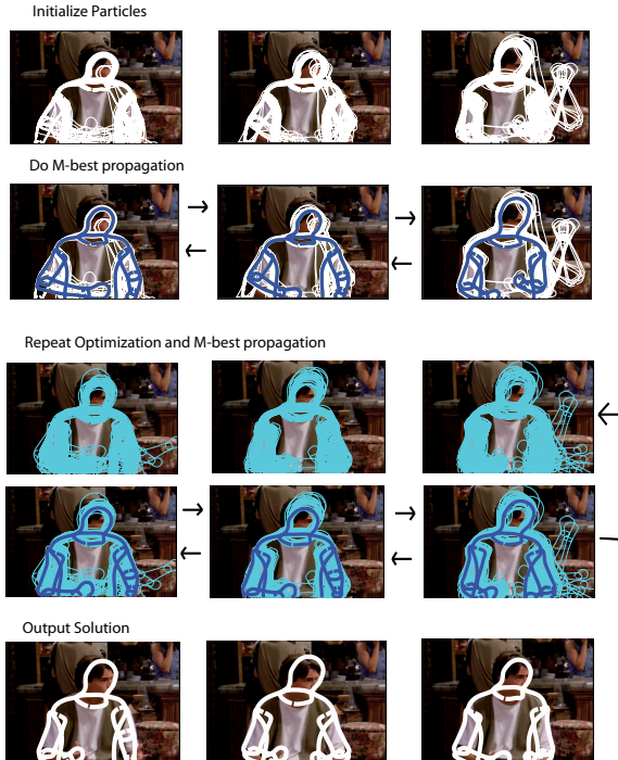
Figure 6. Particle-based optimization. Particles are initialized on each frame (first row), then the M best are propagated through the flow forward and backward (second row). For a defined number of iterations particles are then locally optimized, then the M best are propagated to the neighbors (third and fourth row). Then the best particle on each frame is returned as the solution (last row).
