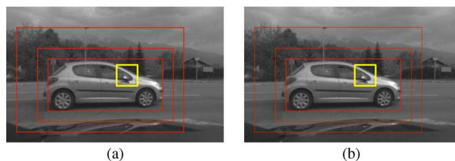
Fig. 2. Possible detection scales from a local feature. (a) Only intensity information is used. The distance of the detection cannot be accurately determined, resulting in false-positive detections at inconsistent distances. (b) Fusion of depth and intensity information. Depth information is used to weigh the possible detections. Detections with inconsistent distances receive a lower weight.
