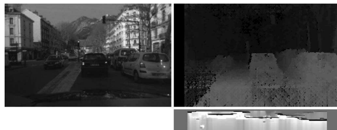
Fig. 4. Occupancy grid computed from stereo vision. (Left) Left image of the stereo pair. (Right) Disparity image computed with the SGM algorithm. (Bottom) Occupancy grid computed in the u -disparity plane.
