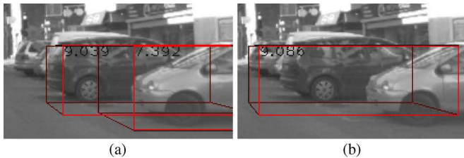
Fig. 13. Comparison of a vehicle detection with and without occlusion reweighting. (a) The evidence is reweighted in order to account for the occluded parts of the objects. This results in accurate detections, although large parts of both objects are occluded. (b) When no reweighting takes place and keeping the same evidence threshold, only one local maximum is found, which results in one detection with inaccurate position.
